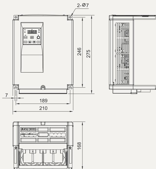
N700E-150LF/150HF, N700E-185LF/185HF, N700E-220LF/220HF
